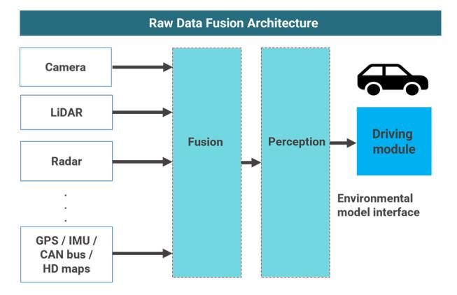
Sensor fusion is a sophisticated technique that integrates data from multiple sensors to create a comprehensive and accurate representation of the environment. The primary objective of sensor fusion is to enhance the reliability and robustness of the data by leveraging the strengths of different sensor modalities. The principles of sensor fusion revolve around combining data streams in a manner that maximizes information content while minimizing ambiguities and inconsistencies.
